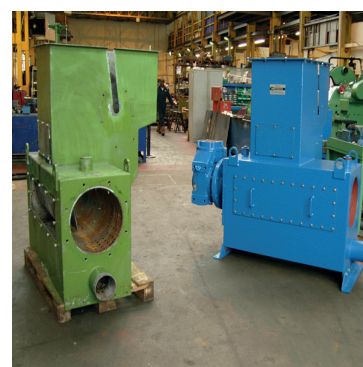
Wash Unit Refurbishment
