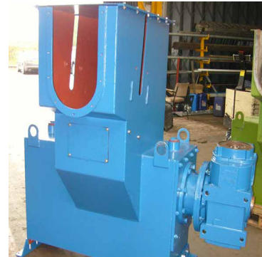
Wash Unit Refurbishment
