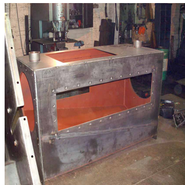
Compactor Body Refurbishment
